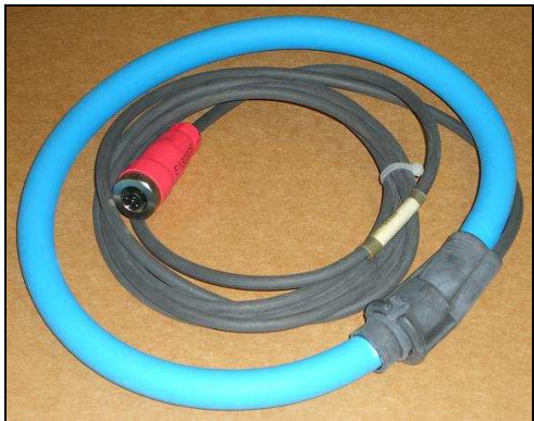
Figure 14 Flexible CT, 3000 Amps
